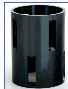
Keystone slot Cut under a 6° angel, this V-shaped slot is non-clogging.
